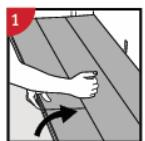
Separate the whole row by carefully lifting up and release the whole row.
