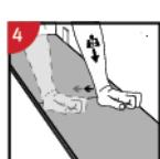
Afterwards press slightly along the short end just installed.
