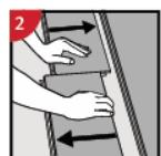
Disassemble the panels by sliding the short ends horizontally.
