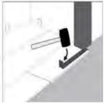
**Step 2**: Use hammer and pull bar to draw in and lock short end of plank.
