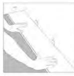
**Step 1**: Begin installation working from left to right. Insert 1/4" wide spacers at ends and edges where planks meet wall.
