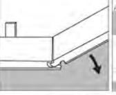
**Step 2**: Lock short end of plank by inserting tongue into groove at an approximate 30 degree angle and drop into place. Continue this process throughout the installation.
