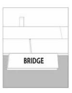
Step 6: Attach a scrap piece of floor to bridge the gap between ends of planks.
