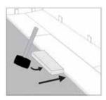
Step 5: IMPORTANT! Use a hammer and tapping block to tap the long edge of the plank to ensure a tight fit. Note: Tapping block should be a minimum of 10" to 12" long. It is important to note that any/all gapping can/will compromise locking system.
