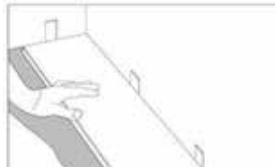
Step 1: Begin installation working from left to right. Insert 1/4" wide spacers at ends and edges where planks meet wall.
