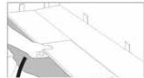
Step 4: Lock long edge of plank by inserting tongue into groove at an approximate 15 degree angle and drop into place. Next slide toward end of previously installed plank until the tongue touches the groove.
