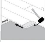
Step 7: Tap end of plank with hammer and tapping block to lock ends of planks together. Remove support bridge and continue with this Step 8: Use hammer and pull bar method until you have completed installing the row. Note: BE SURE TO TAP ON EDGE OF VINYL SO AS NOT TO DAMAGE LOCKING PROFILE.
