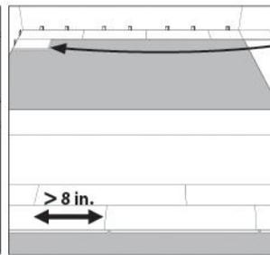
**Step 3:** Use the remaining plank from your cut piece to begin the next row (you will repeat this process throughout the installation). Note: It is recommended that you space end-joints by a minimum of 8 inches.
